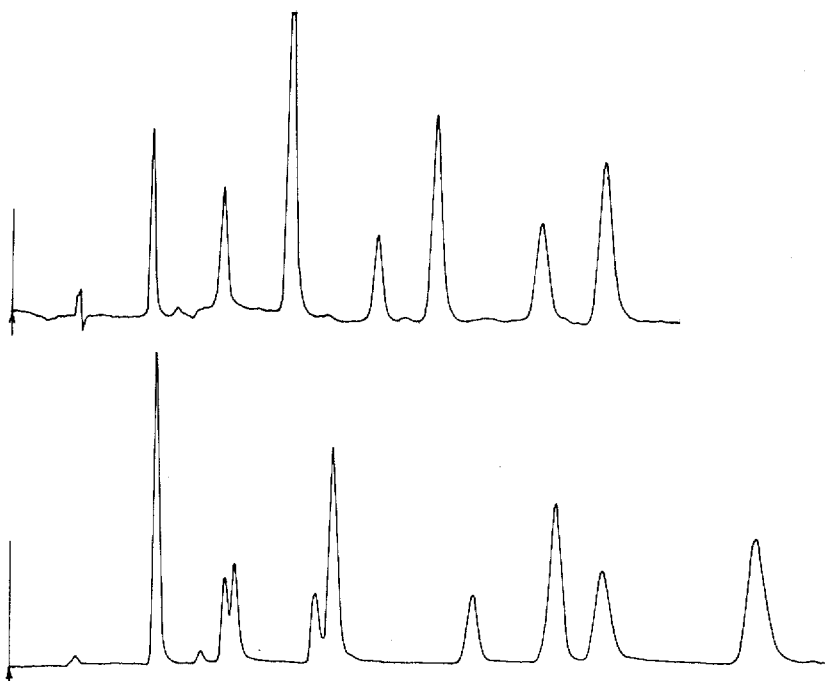
Fig. 2. Chromatogram obtained with a Varian LC 5020 instrument with 25 \times 0.46 cm I.D. columns packed with spherical 5- \mu\text{m} ROSiL derivatized with octyldimethylchlorosilane (above) and octyltrichlorosilane (below). Both phases end capped. Chromatographic conditions and sample as in Fig. 1.
